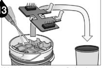
Using a hand tool such as a flat-head screwdriver, detach the PCB from the unit.
