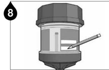
Note the installation date and the scheduled date of lube cycle completion on the label of the Pulsarlube E. Note Please note there is a delay before the actual dispensing
