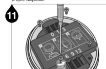
Unscrew the screws to remove the battery cover.
