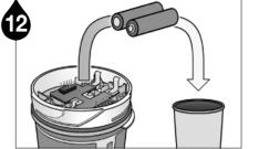
Remove the batteries.
