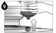
When the selected dispensing period of the Pulsarlube E has completed, remove the lubricator from the application.
